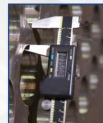
The tubesheet is the most critical component in any scotch marine type boiler and Superior's tubesheets exceed the ASME code thickness by 25% in low pressure units and 33% in high pressure units. Thick tube sheets coupled with tubes 10% thicker than ASME code requirements and 3/4" ligament spacing give Superior Boiler Owners more tube seating surface and long equipment life.
